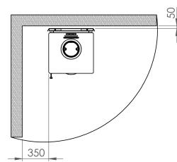
Trinity 1-Eco insulated flue, with optional heat shield.
