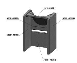
Trinity 3-Eco glass refactory panels parts diagram:
