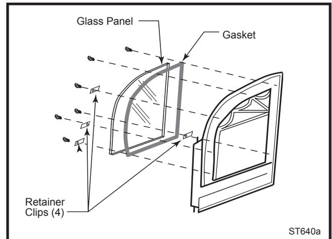
Fig. 29 An exploded view of the glass assembly for the left door.
