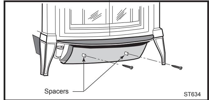
Fig. 15 Use spacers and screws to position the ashdoor heat shield.
