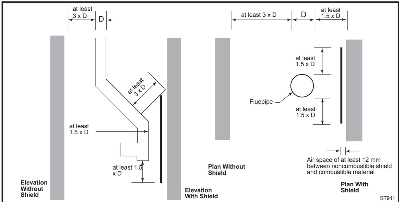
Fig. 13 Connecting fluepipe clearances.
