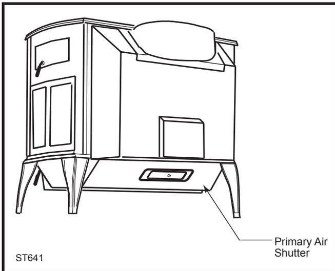
**Fig. 30** The primary air shutter must move freely.
